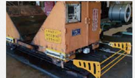
Inductive stop devices for steel coil trolleys
