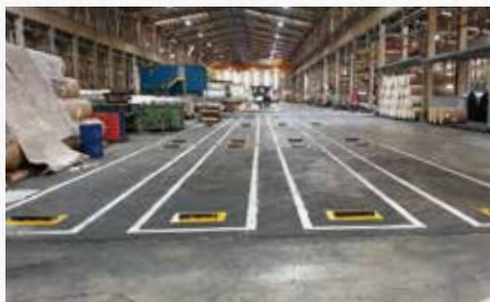
Implementation of controls for steel coil storage
