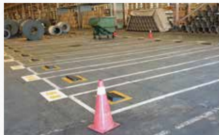
Implementation of controls for steel coil storage
